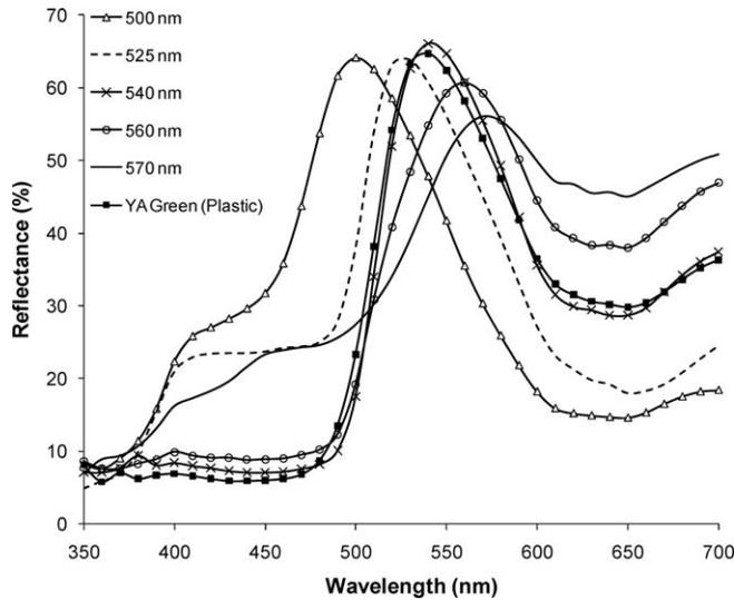
Fig. 2. Reflectance spectra of green painted and plastic traps used in a wavelength comparison study.
