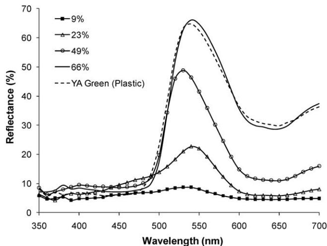
Fig. 3. Reflectance spectra of green painted and plastic traps used in a reflectance comparison study.
