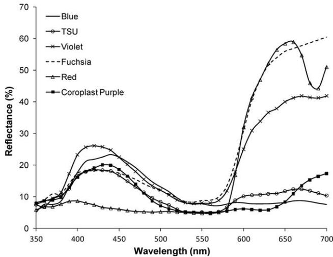
Fig. 1. Reflectance spectra of purple painted and plastic traps.
